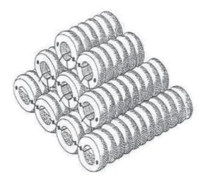
Fig. 5. An artificial habitat that successfully recruited Mediterranean slipper lobster, *Scyllarides latus*. The man-made structure was made of used car tires (32 cm inner diameter, 65 cm outer diameter and 17 cm tire width) connected with 18 mm steel bars and weighted with concrete poured into the lower part of the first row of tires (from Spanier *et al.* 1988, used with permission)
